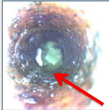
Arthroscopy shaver hand -piece with significant internal corrosion
