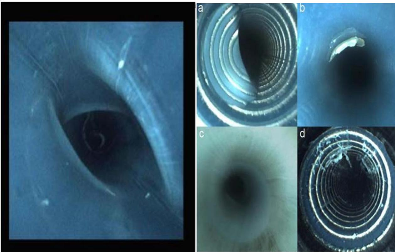
Instrument channel inspection findings: a) retained fluid in a colonoscope. B) debris in a linear echoendoscope. C) staining and discoloration in a duodenoscope. d) scratches and shredding in the bending section of a gastroscop.
